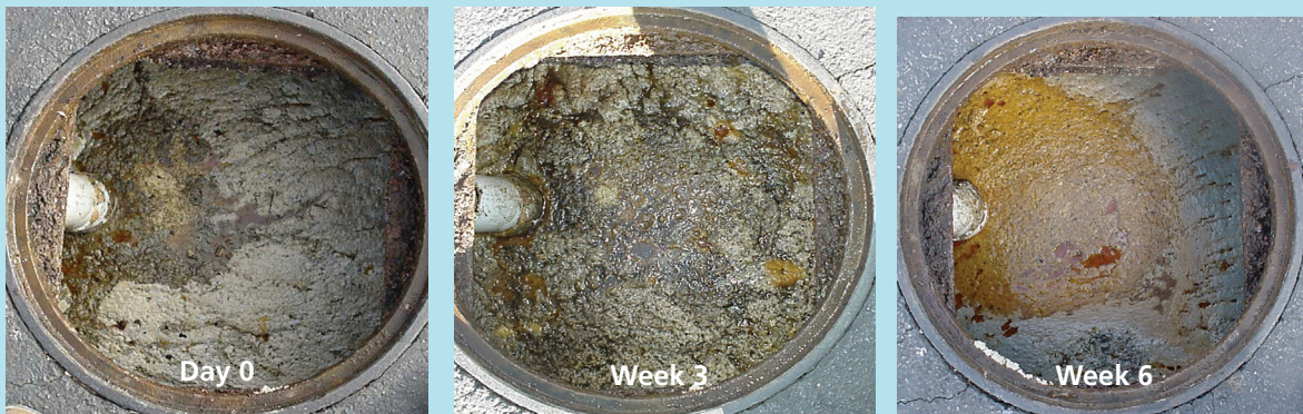
Fig. 1. Novozymes Grease Guard™ contains a patented Bacillus microorganism capable of degrading long-chain fatty acids in low-pH conditions, which can help reduce or slow the buildup of grease in the system over time. These pictures show the progression of treatment with Grease Guard over a 6-week period. The grease layer initially appears thick and heavy, but by week 6 is noticeably thinner and lighter.
